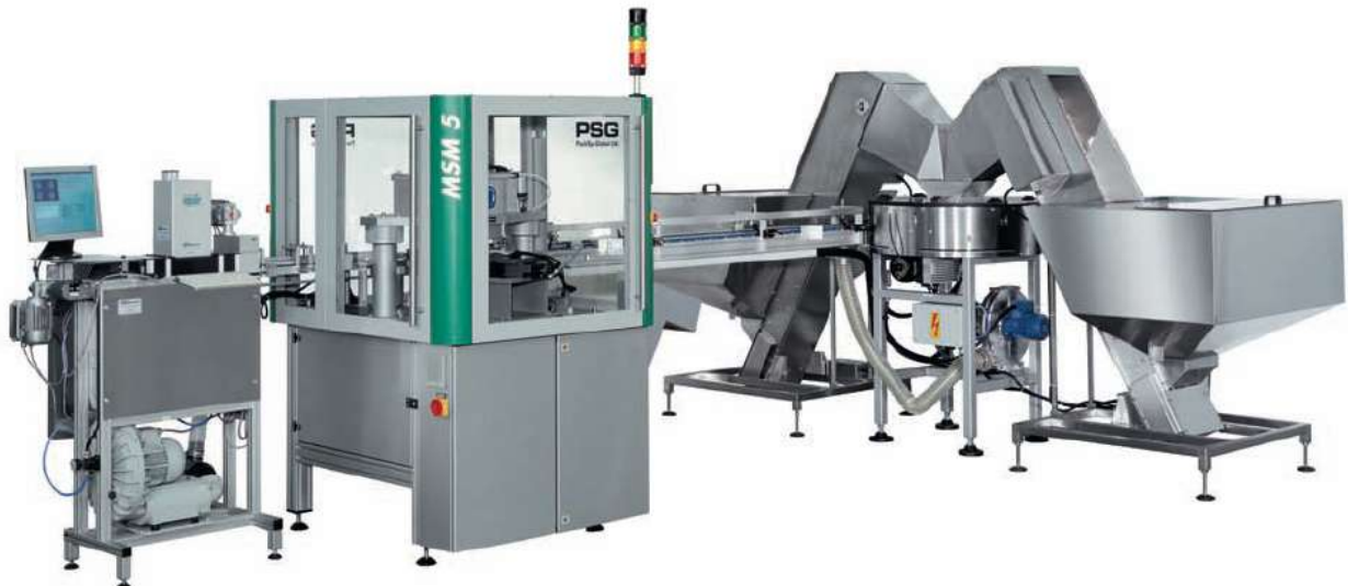
The opsis CAPchecker® in standard configuration, installed in the PSG Slitter Machine at PackSys Global, Switzerland,
